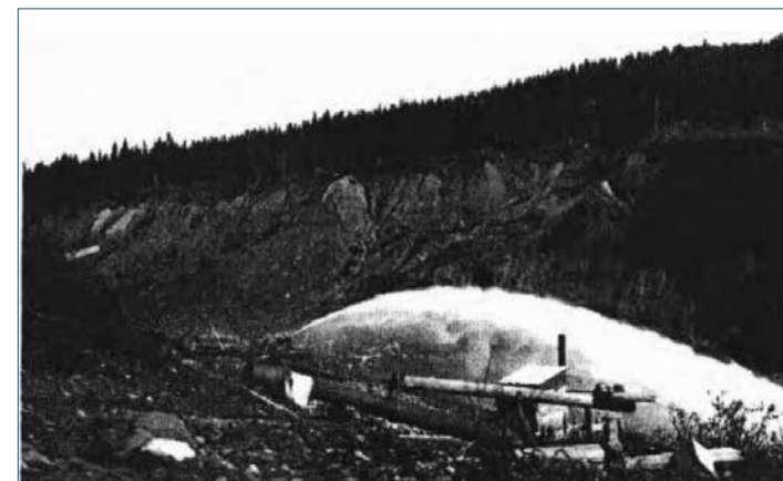
4b. An active hydraulic monitor along the face of the Ketch Mine on the south side of Slough Creek.
